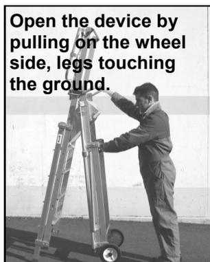
Open the device by pulling on the wheel side, legs touching the ground.
